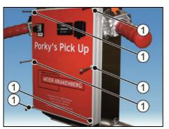
• Loosen bolts (1) of control panel.
