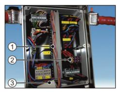
• The control panel (3) can be left hanging on the wiring harness (1) to have free access to the fuse block (2).
