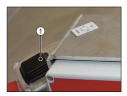
Operate the button ROLLER DRIVE UP/DOWN and set to UP position. Keep the button in that position
