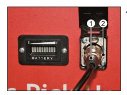
• Connect the charger plug (1) of the charging device to the charger socket (2).
