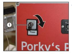
Set key switch POWER ON/OFF (1) to position ON (see illustration).
