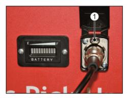
Remove charging device by pressing down the lever (1) slightly and by unplugging the charging plug.
